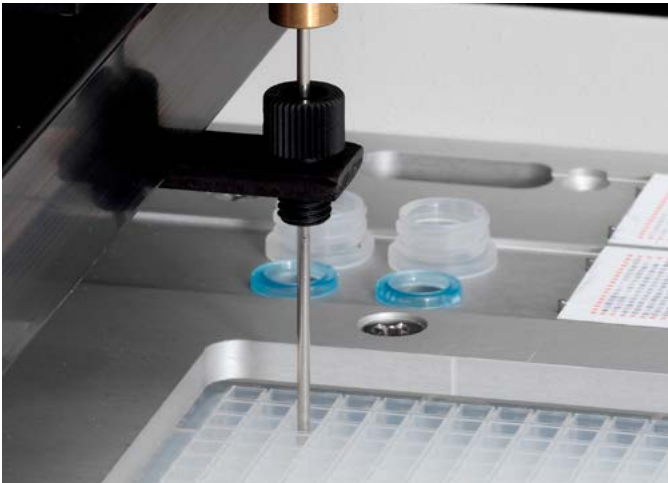
Dissolved peptide-cellulose conjugates in 384 well being spotted onto CelluSpots slides.
