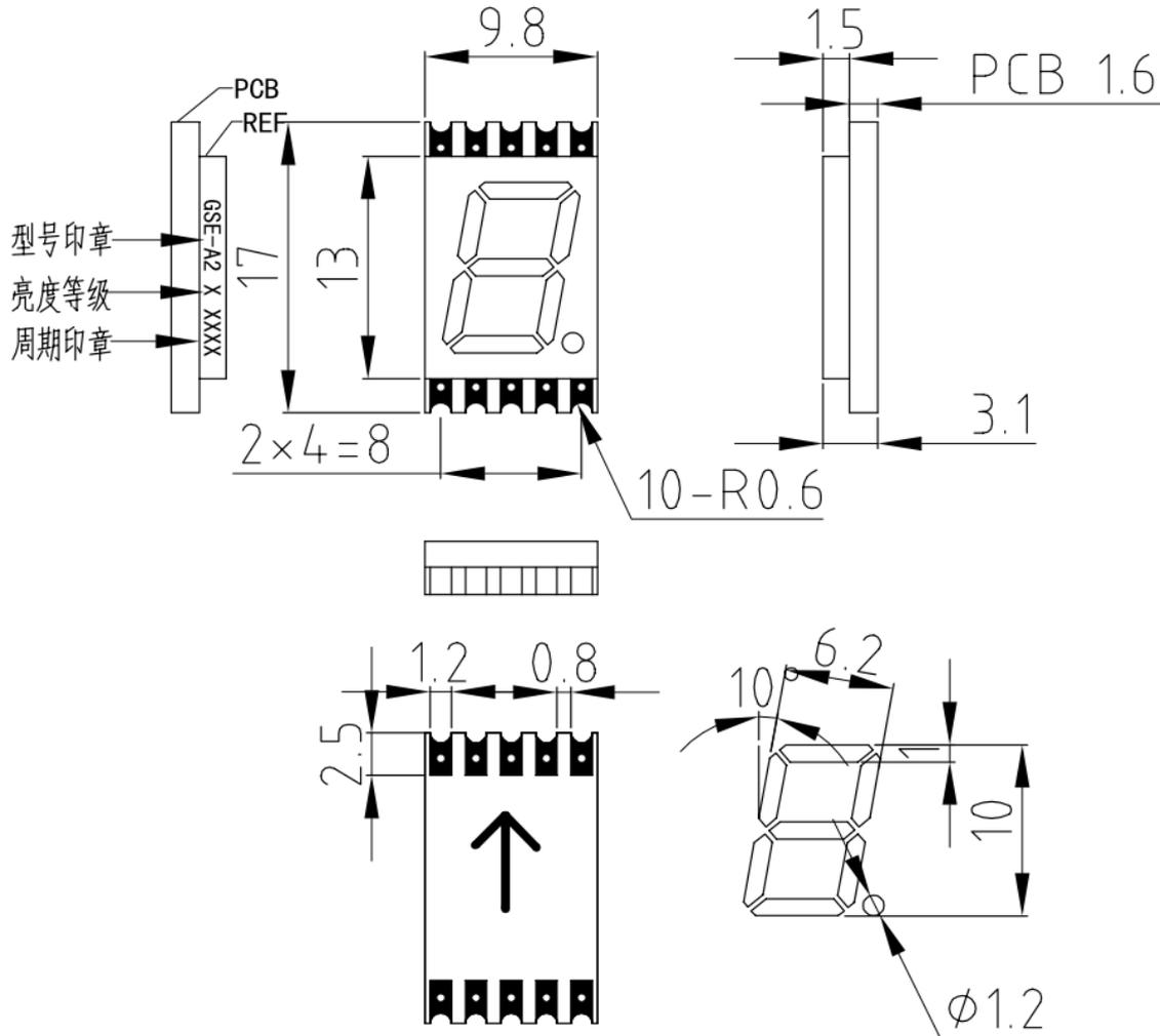
NOTES : All dimensions are in millimeters (inches) tolerance are  $\pm 0.25\text{mm}(0.010)$  unless otherwise noted
