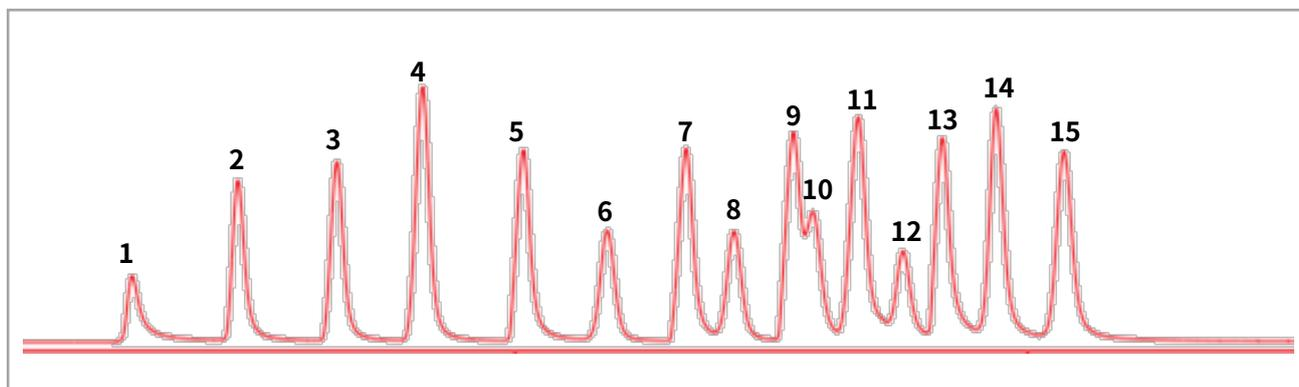
**Fig 4. chromatogram of oxygenates using D4815 qualitative ID mix standard (47213)**
