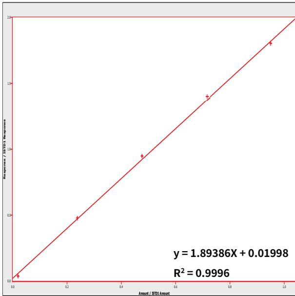
**Fig 5. calibration curve of *tert*-amylalcohol**
